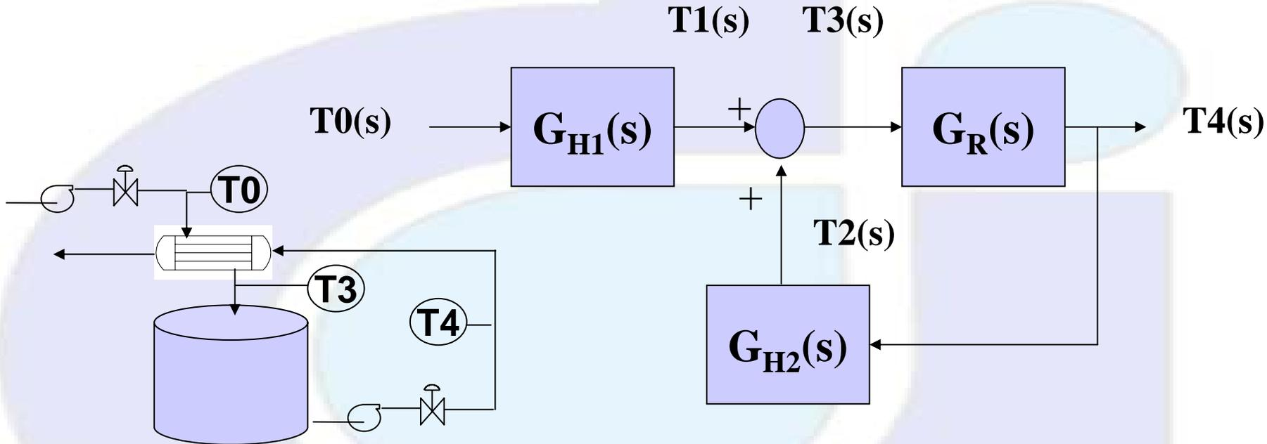
$$\frac{T_4(s)}{T_0(s)} = \frac{G_R(s)G_{H1}(s)}{1 - G_R(s)G_{H2}(s)}$$
