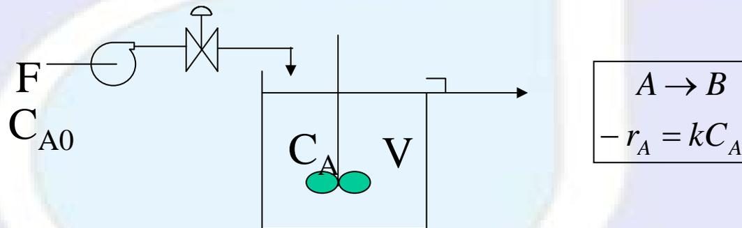
$$\tau \frac{dC_A}{dt} + C_A = KC_{A0} \quad \text{con} \quad \tau = \frac{V}{F + kV} \quad \text{y} \quad K = \frac{F}{F + kV}$$
