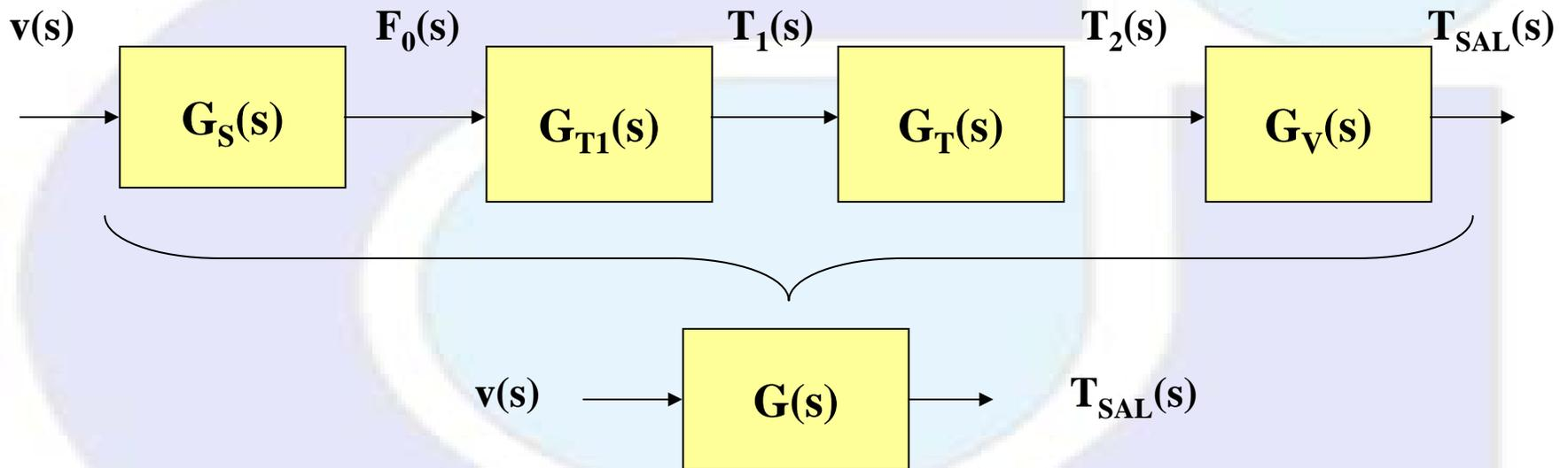
$$\frac{T_{SAL}(s)}{v(s)} = G(s) = \left[ \frac{T_{SAL}(s)}{T_2(s)} \right] \left[ \frac{T_2(s)}{T_1(s)} \right] \left[ \frac{T_1(s)}{F_0(s)} \right] \left[ \frac{F_0(s)}{v(s)} \right]$$
